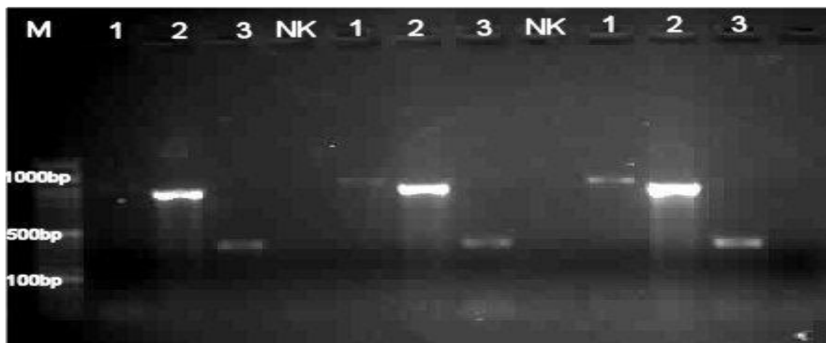
Figure 3. Gel images at different primer concentrations (from left to right: 0.6, 0.8, and 1 µL primer concentrations)
