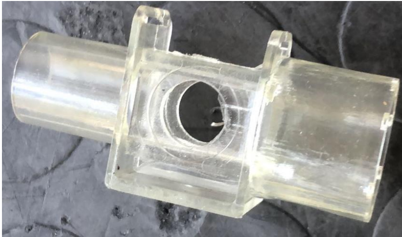
Figure 3. Custom-designed mainstream airway adapter manufactured from polycarbonate using a dedicated mold used in the developed capnometer prototype
