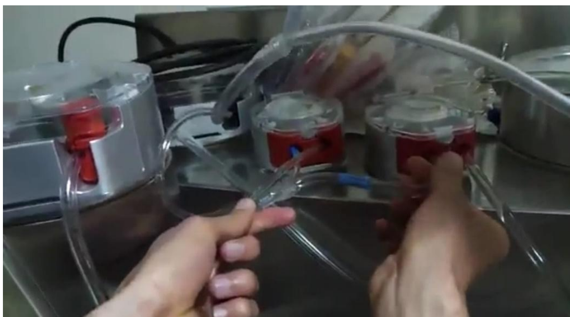
Image 1. Mini pumps and line coupling with y-connection.
